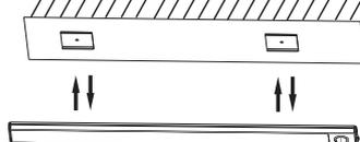
4. After installation, the light is magnetically attached on the metal clip and can be taken off at any time.
