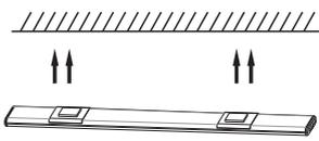
3. Attach the cabinet light with metal clips to the surface of the target position.
