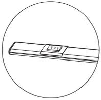
1. Paste the double-side tape to the back of the metal clip.
