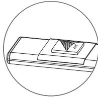
2. Peel off the protective films on the double-side tape.
